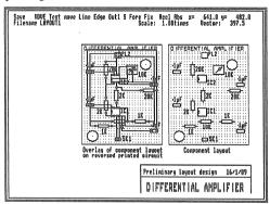
Superimposing an image of a printed circuit board
